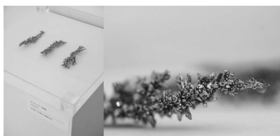
Fig. 4 Dendritic titanium crystals produced by molten salt electrolysis are displayed as design/artistic products. ( http://www.design-lab.iis.u-tokyo.ac.jp/exhibition/rp01/ ) (Photo by courtesy of Mr. Yashushi Kato)
