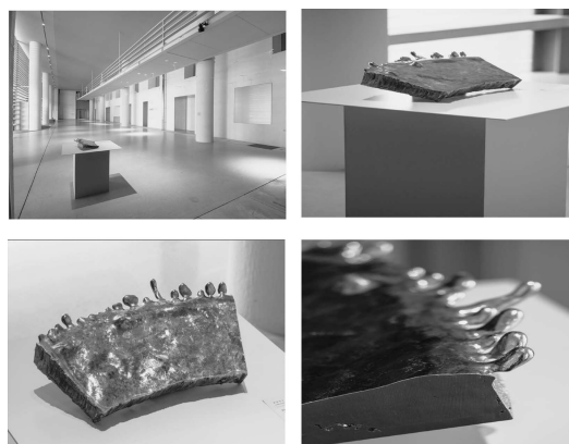
Fig. 6 Top portion of a titanium ingot produced after electron beam melting. (Photo by courtesy of Mr. Yasushi Kato)
