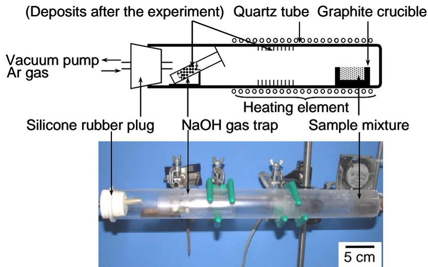
Figure 3 Experimental apparatus for the chlorination of titanium granules using  $\text{FeCl}_2$ .
