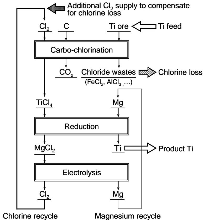
Figure 1 Chlorine cycle in the Kroll process.
