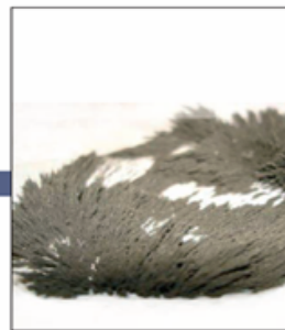
Drying fine-grained iron in rotating magnetic field
