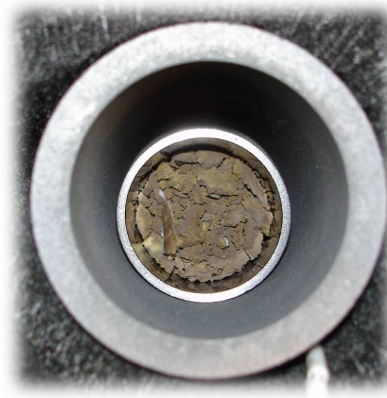
Prior to re-melting: Deposit in glassy carbon crucible placed in induction furnace
