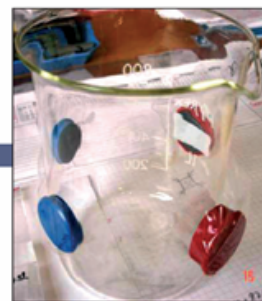
Beaker with fixed magnets on the outside
