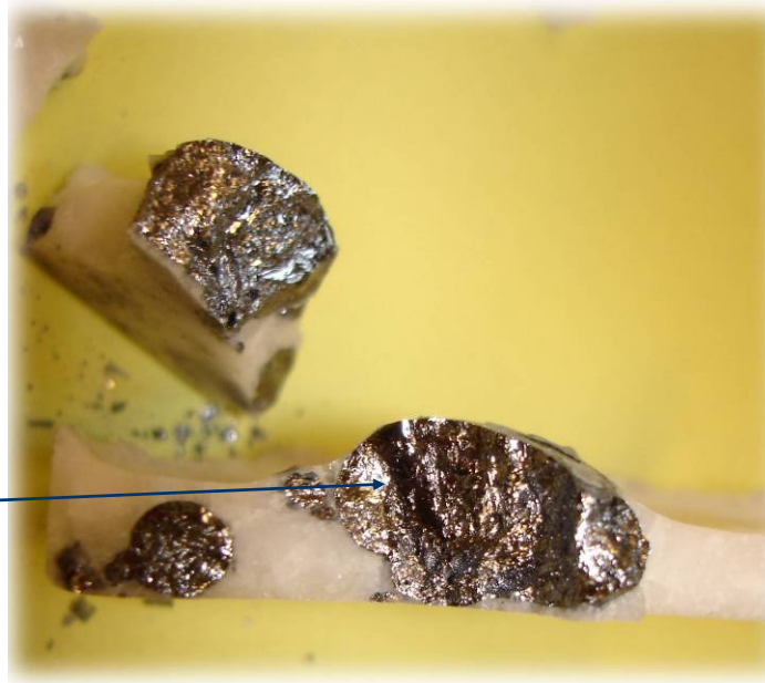
Broken globule of silicon that could easily be separated from the frozen flux.
