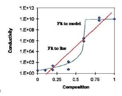
Composite conductivity should behave according to the McLachlan Equation. Fitting the parameters of this equation with gives a completely curve fit than an linear approximation. iSIGHT datamatching component enables this application. Dr. Julie Runyan, Dr. Rosario Gerhardt GT
