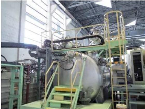
Apparatus of electron beam melting
