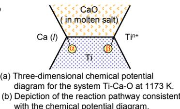
Fig. (a) Three-dimensional chemical potential diagram for the system Ti-Ca-O at 1173 K. (b) Depiction of the reaction pathway consistent with the chemical potential diagram.
