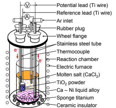
Fig. Schematic illustration of experimental apparatus for TiO<sub>2</sub> reduction using the EMR.
