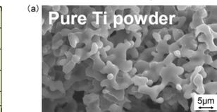
Pure titanium powder was obtained using the EMR.
