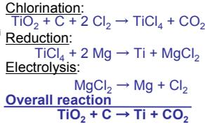
At present, titanium is manufactured by the Kroll process.
