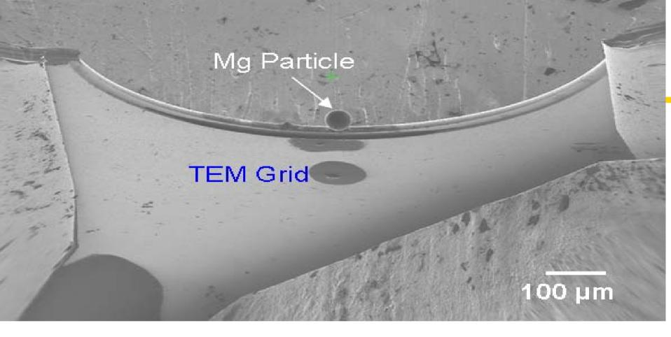
A Mg particle is mounted onto the edge of the TEM grid using an external lift-out tool
