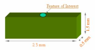
Sample mounted on a TEM grid After carefully polished by a tripot polisher
